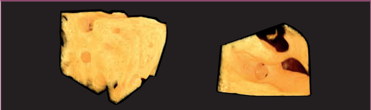
Figure 7: Micro CT 3D image of Bioscaffold regenerated bone sample @ 1 \mu\text{m} resolution
